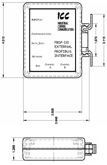
Figure 1: Enclosure Dimensions (units are inches)
